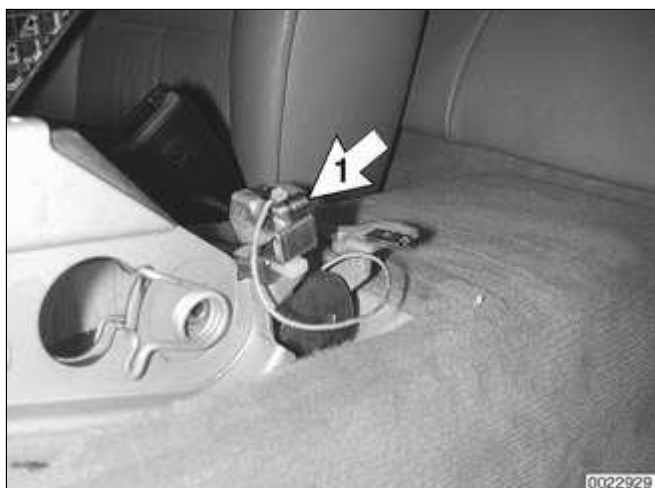
◀ Fig. 49 Under center console, rear of parking brake handle 1 - Parking brake warning switch
